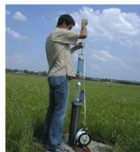
Ground water sampling
