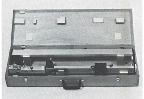
The tracking device TRA2 is designed to fulfil the condition. Once the photographs are oriented as mentioned above, the MS27 can be displaced to all the parts of the overlap without any rotation, thus keeping the vertical parallax imperceptibly small.
